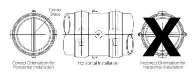
• For horizontal installations, the center brace inside the Series W715 AGS Double-Disc Vic-Check Valve must be in the vertical position, as shown above.
